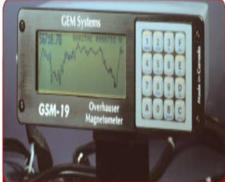
**Overhauser (GSM-19W) Walking Magnetometer console. Can also be configured with additional sensor for gradiometer (simultaneous) readings.**
