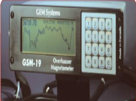
**Overhauser (GSM-19W) Walking Magnetometer console. Can also be configured with additional sensor for gradiometer (simultaneous) readings.**
